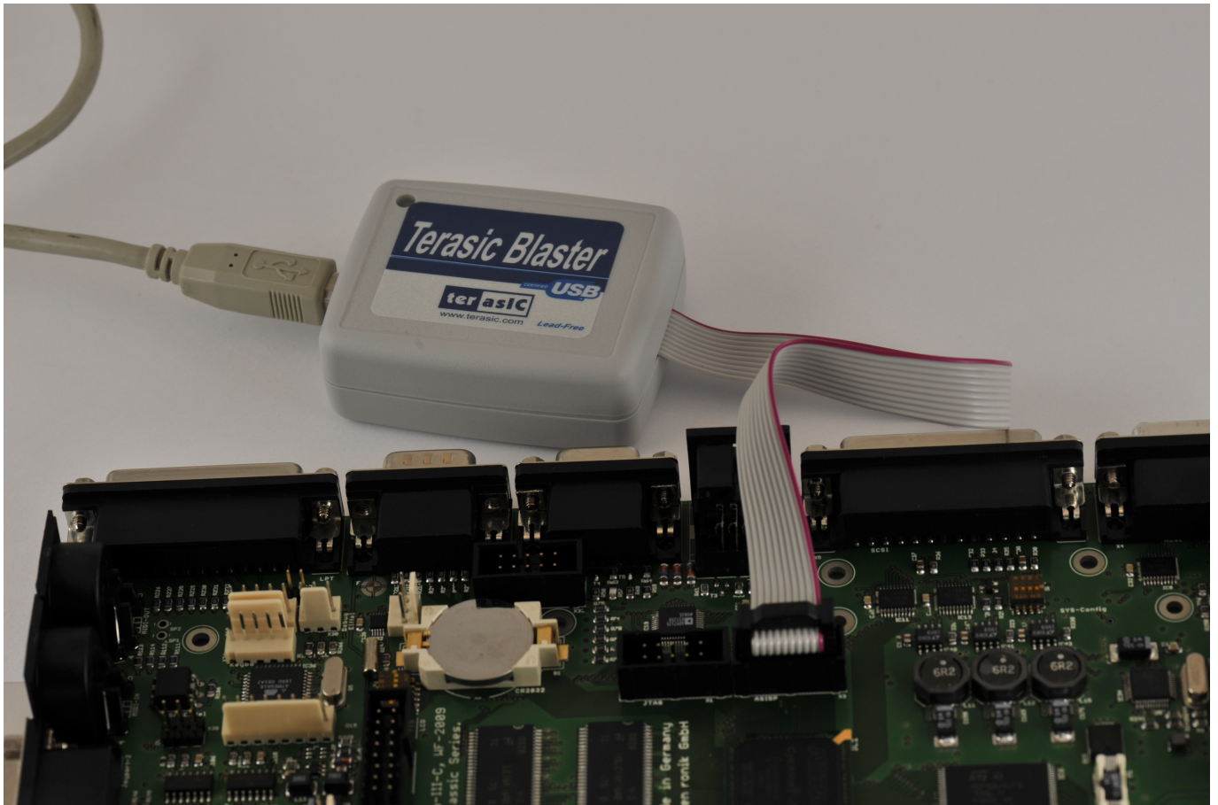
Figure 20: Connecting a USB Blaster to the Active Serial Interface.
