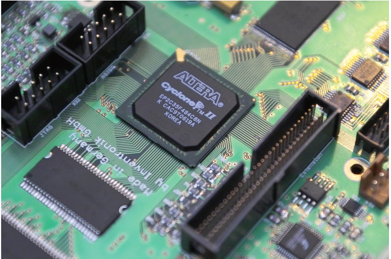
Figure 1: The heart of the Suska-III-C: Cyclone-II FPGA device
